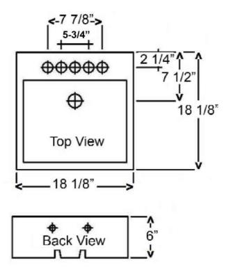
Dimensions of fixture are nominal and may vary within the range of tolerances established by ANSI Standard A112.19.2-2018. Dimensions and specifications subject to change without notice.
